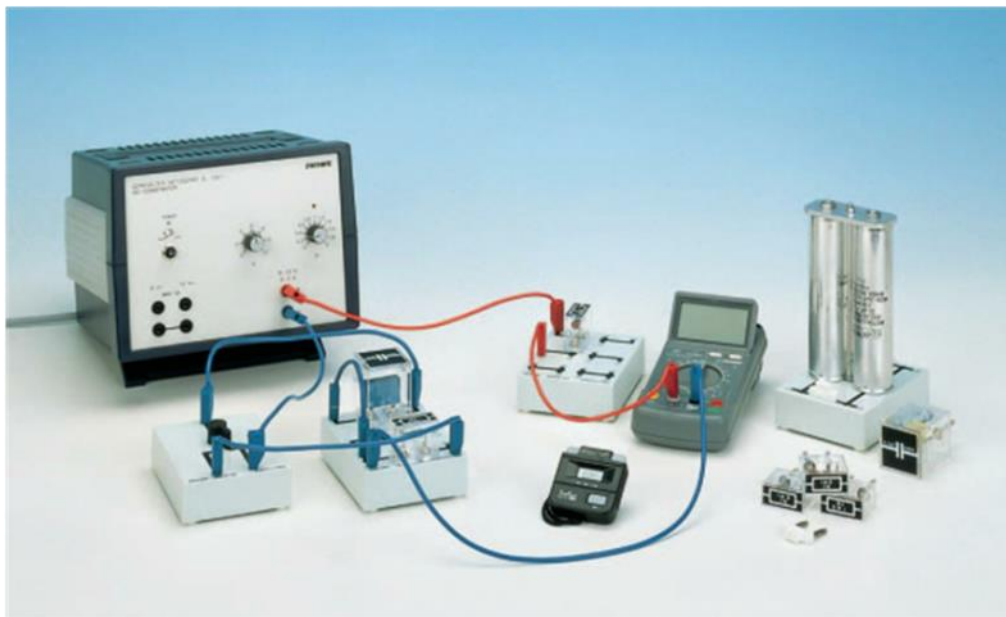
Figure 7-2 Capacitor discharge setting up the testing apparatus
